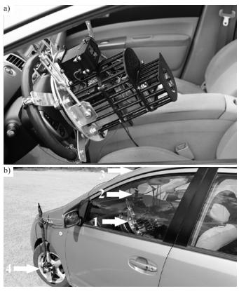
Fig. 2. Experimental research: a – automated steering device mounted on the test vehicle; b – autonomous test vehicle with 1 – automated steering device, 2 – GPS tracker; 3 – GPS antenna, 4 – angular velocity sensor
