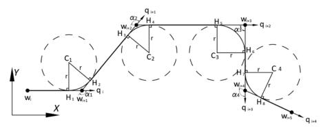
Fig. 1. Scheme of path re-planning using the vector based Dubins path approach
