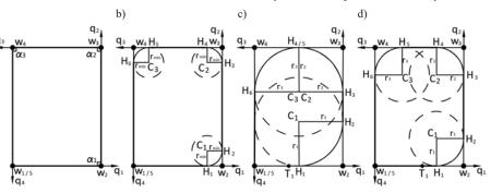
Fig. 3. Basic schemes of the predefined and re-planned paths: a – the predefined path; b – the path re-planned while using the non-modified Dubins path approach; c – the path re-planned while using Eq. (14); d – the path re-planned while using Eq. (17)
